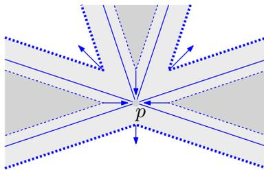
Fig. 2. A wavefront before (dotted), at (solid), and after an event (bold), with blue arrows showing movement direction of wavefront vertices. The *standard pairing technique* for handling a split event pairs each edge with its neighbor in the cyclic order with which it was not paired before (color online).
