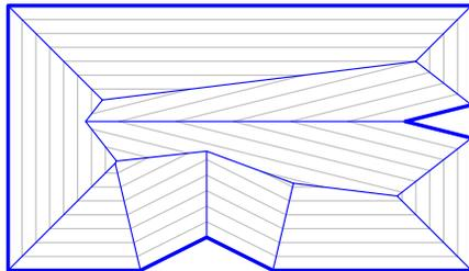
Fig. 1. The straight skeleton  $\mathcal{S}(P)$  (blue) of a polygon  $P$  (bold) is defined as the traces of wavefront vertices over time. Instances of the wavefront  $\mathcal{W}_P(t)$  at different times  $t$  are shown in gray (color online).
