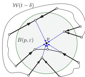
Fig. 8. A multi-split event occurs at location  $p$ . The involved edges form four chains. The simplified wavefront  $\mathcal{W}'$  contains exactly eight edges, shown in bold, stemming from those chains.
